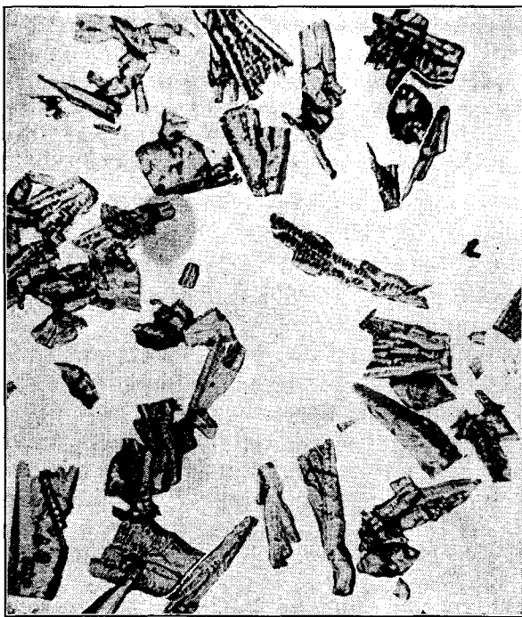
FIGURE 104. Tetracene Crystals (150X).
