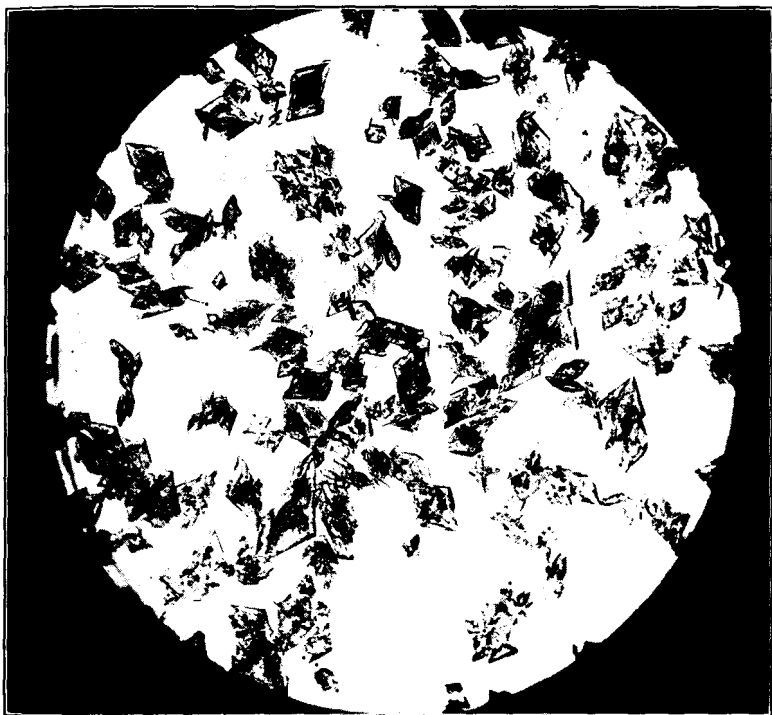
FIGURE 94. Mercury Fulminate Crystals for Use in Primer Composition (30X).
