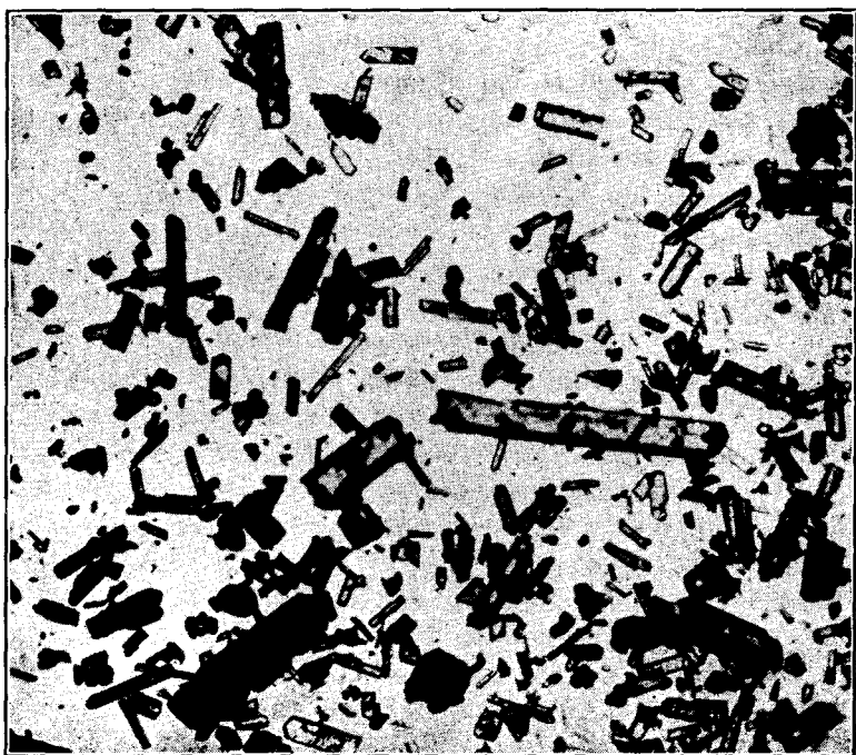
FIGURE 49. Commercial Sample of Ammonium Picrate (25×).
