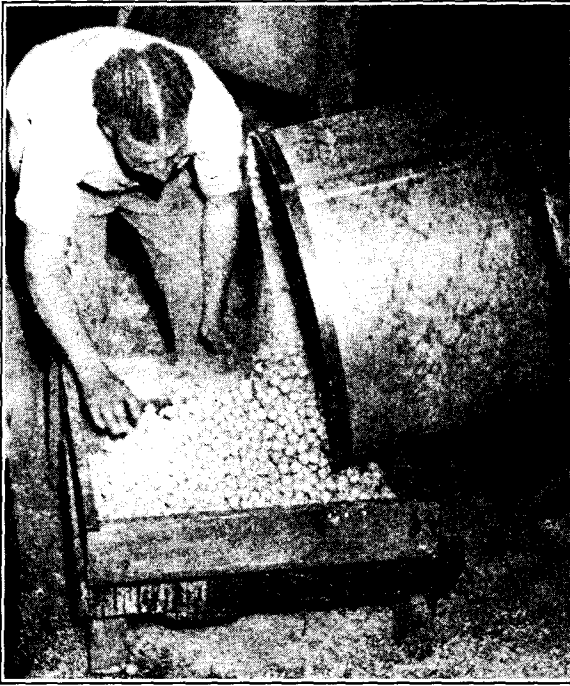
FIGURE 35. Manufacture of Globe Torpedoes. Removing the moist spheres from the tumbling barrel. (Courtesy National Fireworks Company and the Boston Globe .)
