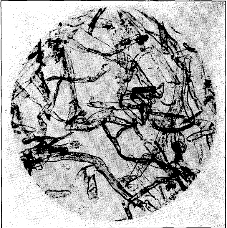
FIGURE 62. Nitrocellulose Fibers before Beating (132 \times ). (Courtesy Western Cartridge Company.)
