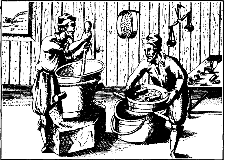
FIGURE 18. Gunpowder Manufacture, Lorrain, 1630. After the materials had been intimately ground together in the mortar, the mixture was moistened with water, or with a solution of camphor in brandy, or with other material, and formed into grains by rubbing through a sieve.
