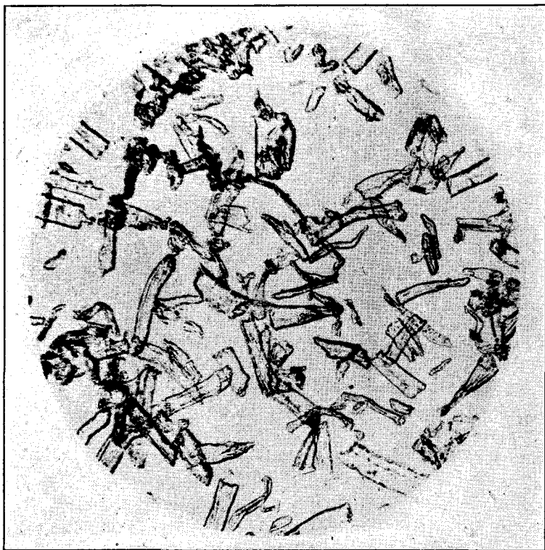
FIGURE 63. Nitrocellulose Fibers after Beating (132 \times ). (Courtesy Western Cartridge Company.)
