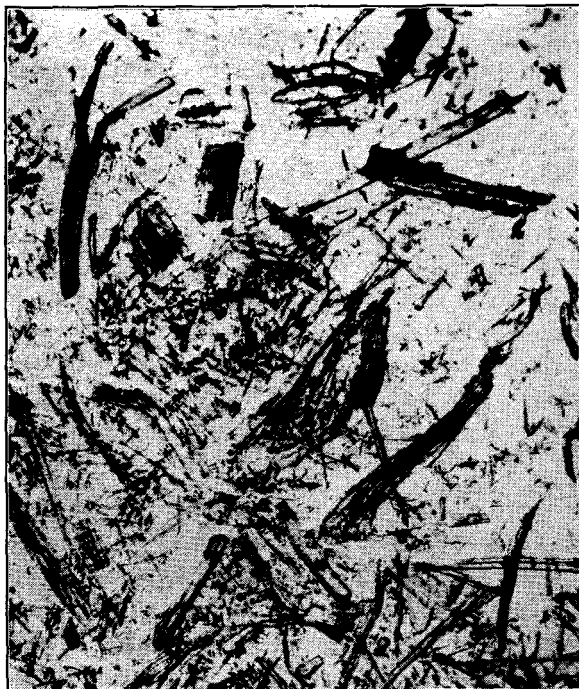
FIGURE 89. \alpha -Nitroguanidine (25 \times ). Small crystals from the rapid cooling of a hot aqueous solution.
