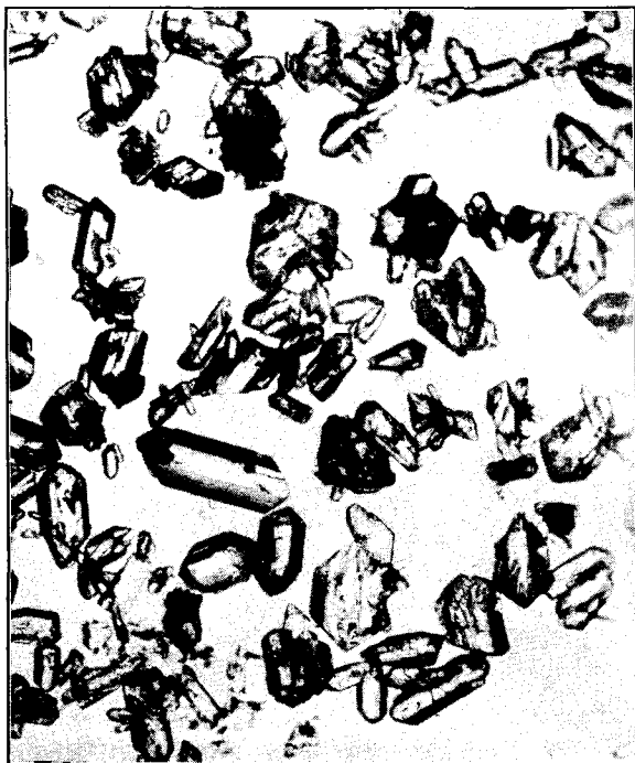
FIGURE 102. Lead Styphnate Crystals (90X).
