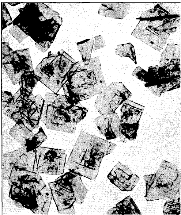
FIGURE 103. Diazodinitrophenol Crystals (90 \times ).
