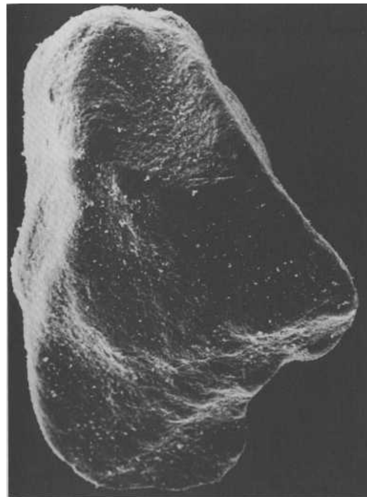
A grain of commercially-produced black powder, magnified 80 times. Extensive mixing and grinding of moist composition produces a homogeneous mixture of high reactivity. A mixture of the same three components-potassium nitrate, sulfur, and charcoal-that is prepared by briefly stirring the materials together will be much less reactive. (J. H. McLain files)
