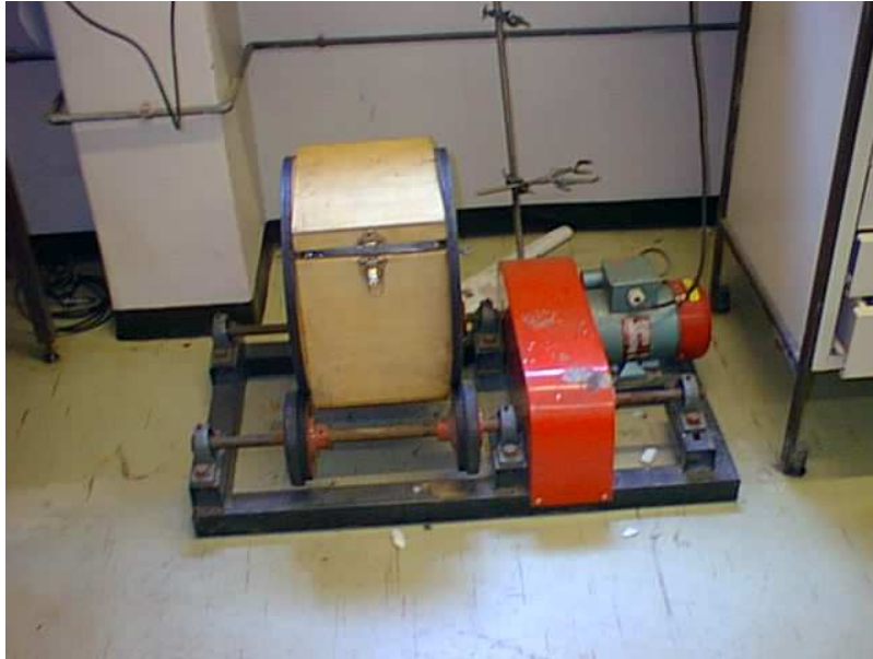
Figure 6-1: Equipment used for Tumble Mixing of Compositions (Tumbler)
