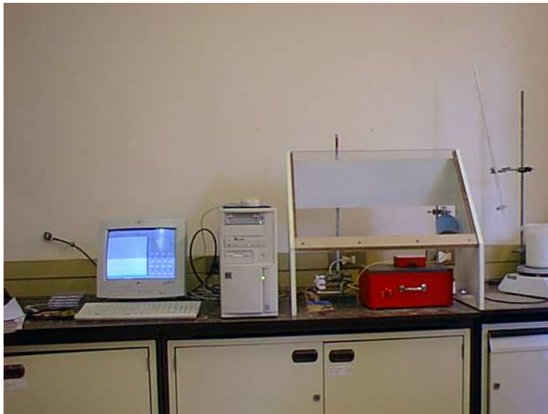
Figure 6-8: Data Acquisition Computer
