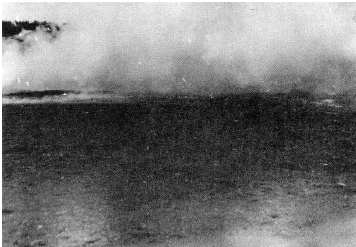
Figure 2-18 Smoke Cloud Produced by Two No 80 Grenades
