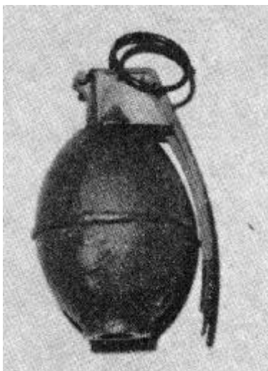
Figure 2-5 Assembled M62 Grenade - (Safety Clip Removed)
