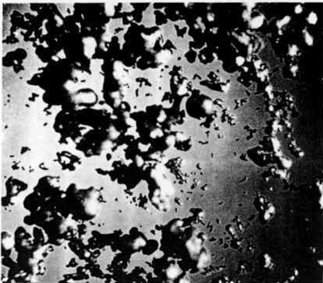
Aluminum: Alcoa 101. This product is useful as a source of very large particles when blending aluminums. The first photomicrograph of this aluminum shows the many fines which are too small and too irregular. This aluminum gives poor spritz in most mixes if used alone. (1mm = 5 microns)
