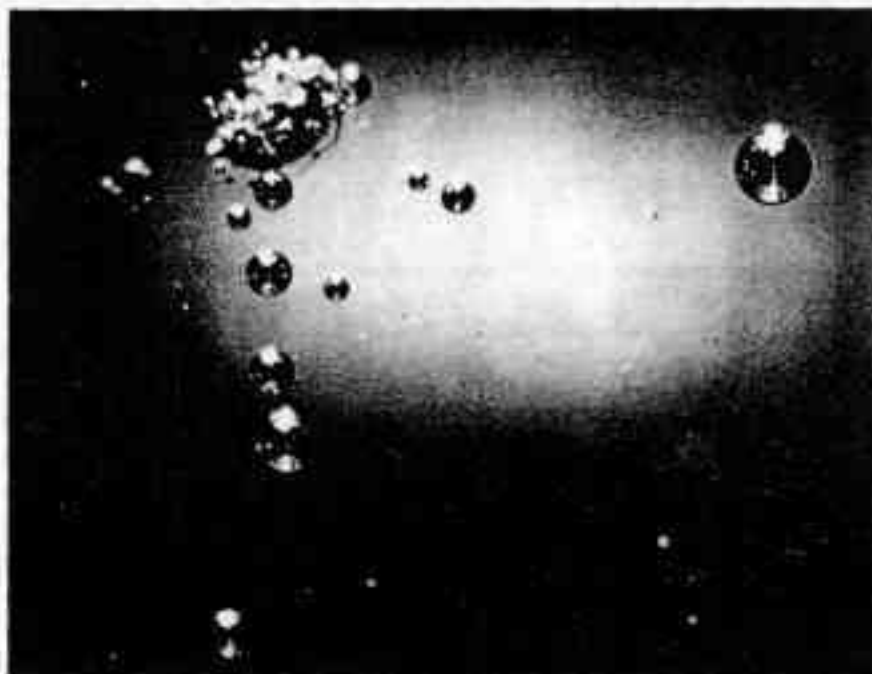
Example of chemical instability of combustion products. Spritzel oil covered in less than two seconds is here evolving gas in less than thirty seconds. Note bubbles of gases. (1mm = 5 microns)
