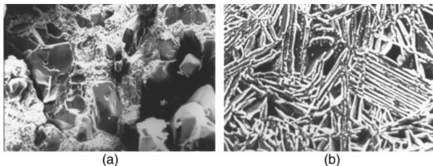
Figure 7-18. Scanning electron microphotographs of RDX composite propellant surface before combustion (a) and after quenching (b) by rapid pressure decay from the burning at 2 MPa.
